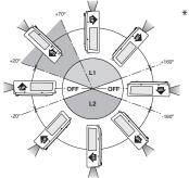
\* When installing the projector in upwardly inclined position, install the projector bottom side up.
